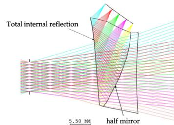
Figure 4. The setup for optical see-through mode.
